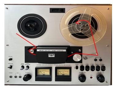
**Step 3:** Thread the tape as per the threading diagram and secure it to the take up reel on the right spindle.
