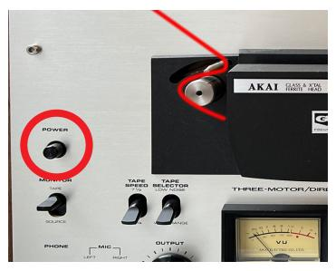
**Step 1:** Plug the power cord into the electrical outlet and turn the power on.
