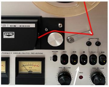
**Step 6:** Use the **Rewind, Stop, Play,** and **Fast Forward** controls on the **Akai** to move the tape.
