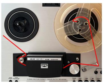
**Step 2** Place the reel of tape onto the left spindle of the **Akai** so that the tape feeds off counter clockwise.
