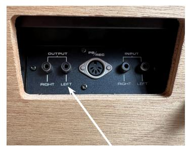
**Step 5:** Connect the outputs of the **Akai** deck to the inputs on the bottom of the **Zoom** recorder (see **Zoom** Instructions).
