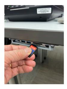
• Once you've removed the SD card from the Zoom unit, insert it into a Mac or PC in order to copy your audio files.
