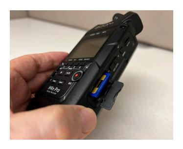
• When you are ready to retrieve your files open the SD compartment door and remove the SD card.
