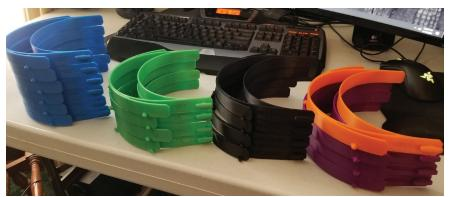
The 3D printers have also been hard at work during the closure, producing face shield head pieces and visor guards, led by an initiative from Technology Librarian Dan Criscione. Volunteers are then using the pieces to
