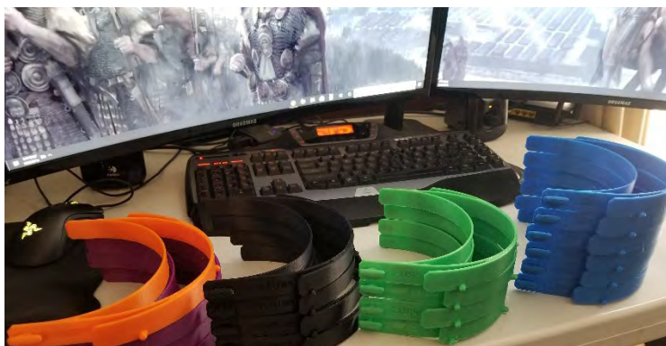
3D printed parts for face shields
